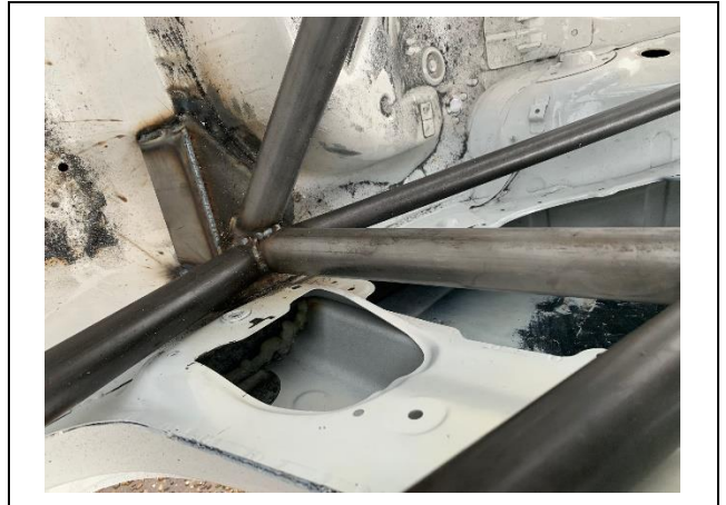
PHOTO 4 MAIN ROLLBAR TO FLOOR ATTACHMENT
