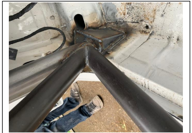
PHOTO 6 FRONT ROLLBAR TO FLOOR ATTACHMENT
