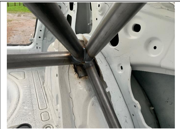
PHOTO 5 REAR BACKSTAY TO BODYSHELL ATTACHMENT
